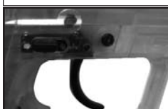
Fig. 2B - Push rearward for "OFF SAFE"
