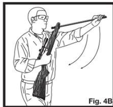
Do not cock your airgun until you are ready to load and fire, since the only way to un-cock your airgun is to fire it. Firing your gun without a pellet in the chamber (dry firing) may cause damage to your airgun.
