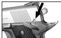
Fig. 2B - Push down for "OFF SAFE"
